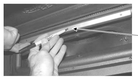
Mark the location of the center hole on the gasket clip.
