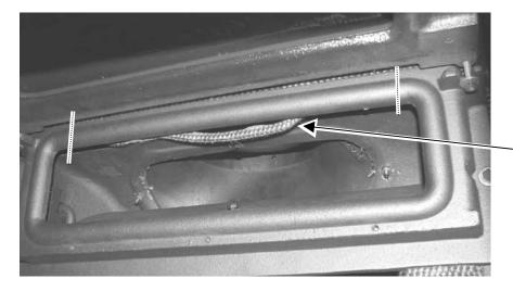
If the gasket is drooping in the center, simply cut the gasket along the dotted lines. Remove the gasket and replace with the included gasket.
