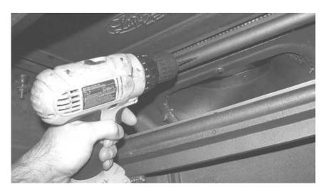
4 Replace the gasket clip (remember to rotate it into place) and secure it with the center screw. NOTE: Do not over-tighten this screw – this may cause the screw head to break off.
