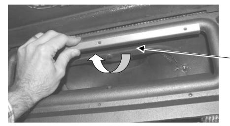
Rotate the clip forward until it is firmly against the cast iron housing.
