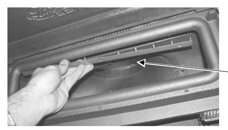
Hold the gasket clip with the pins to the rear, facing upwards. Slide the clip over the bypass gasket – the pins will depress or pierce the gasket.
